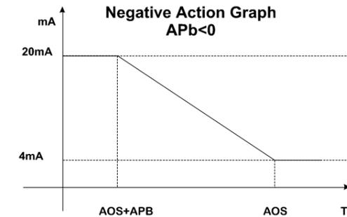
**NOTE:** When the defrost is in progress, the analogue output is set to the minimum value (4 mA). This condition lasts until the defrost terminates.
