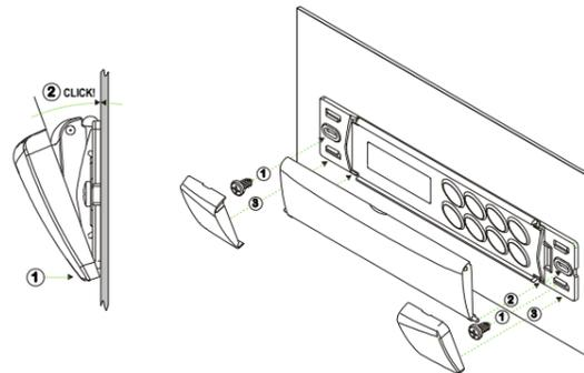
**8.3 MOUNTING WITH KEYBOARD COVER OPENING UPWARD**
