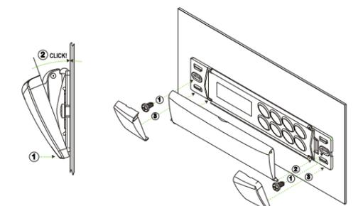
7.3 MOUNTING WITH KEYBOARD COVER OPENING UPWARD
